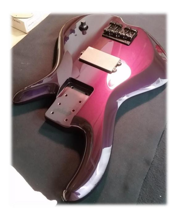
Simplicity is rounded off by fitting an EMG MM style pickup. One single dual pot. Volume and tone thanks-oh and a blue light-so that the owner knows it's 'on'!
